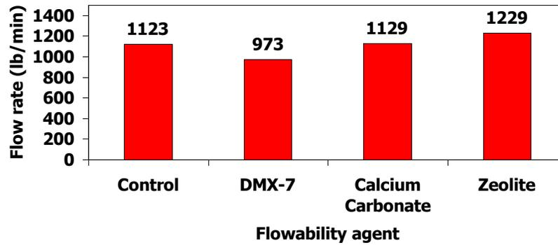
Figure 3. Effect of flowability agents on flow rate of DDGS
