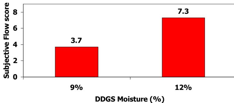
Figure 2. Effect of DDGS moisture content on subjective flow score of DDGS out of a feed truck
