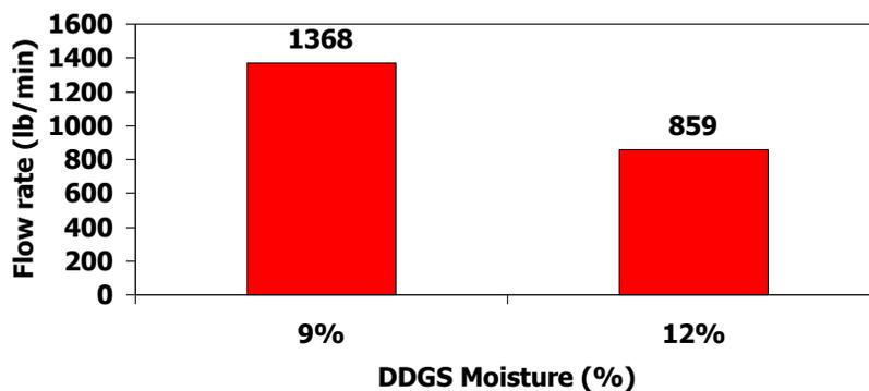
Figure 1. Effect of DDGS moisture content on flow rate of DDGS out of a feed truck
