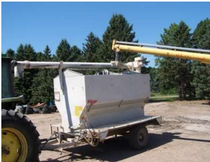
**Figure 3. Feed wagon used to weigh feed for flow evaluations**
