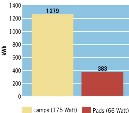
For heat pads, electrical demand was about one-third the amount of the heat lamps, and electrical consumption about one-quarter. The bottom line: Puratone saved approximately \$3 per crate each month in electricity costs with heat pads.
