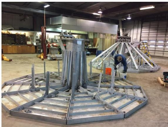
Figure 5. Wind Tower Foundation Assembly
